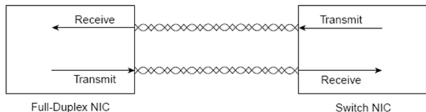
10BASE-T Full-Duplex Operation Using a Switch
